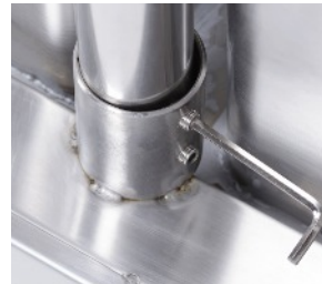
Tighten set screws (2 per leg) securing underframe to sink top DO NOT OVER TIGHTEN
