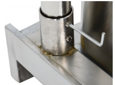
Tighten set screws (2 per leg) securing underframe to sink top DO NOT OVER TIGHTEN
